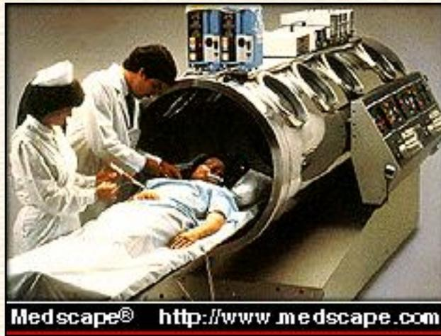
Figure 2. Recent technical innovations have allowed critically-ill patients to undergo therapy in the monoplace chamber. Monoplace chambers are designed for single occupancy. They have a pressure capability of 3 atmospheres absolute and are compressed with 100% oxygen. Reprinted from Hyperbaric Chambers Systems & Management.
